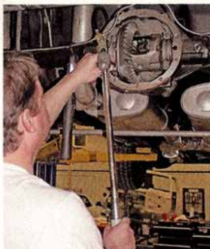
Bryan torqued the carrier caps to 60 ft-lb. Some instructions say snugging the caps is adequate, but he believes it's better to measure with the caps at full load.
