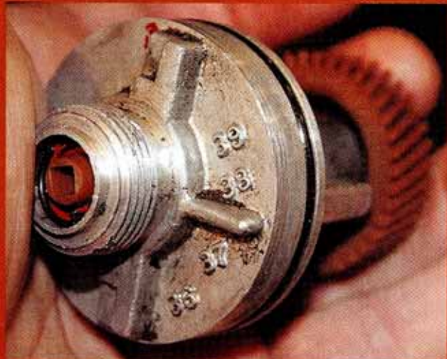
The old gear assembly has the numbers of the driven gears it will accept cast into the case. This assembly is held in place with one bolt and a Y-shaped retainer.
