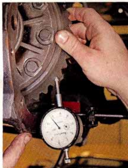
We then took the critical backlash measurement at a few different places on the ring gear. A dial indicator was set on a tooth of the ring gear each time, and the amount of play in the gears was measured. The instructions said to look for a backlash of 0.006-0.010. Ours measured 0.014 so additional shims were needed.
