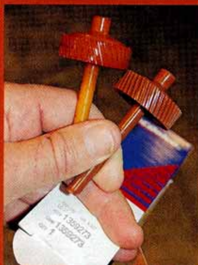
The original driven gear (left) is a natural color, while the replacement gear (right, GM PN 1359273) is brown. The color can be hard to determine unless seen side by side.
