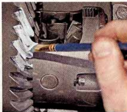
Bryan torqued the carrier caps to 60 ft-lb. Some instructions say snugging the caps is adequate, but he believes it's better to measure with the caps at full load.
